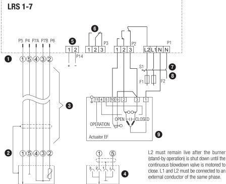
(stand-by operation) is shut down until the continuous blowdown valve is motored to close. L1 and L2 must be connected to an external conductor of the same phase.
